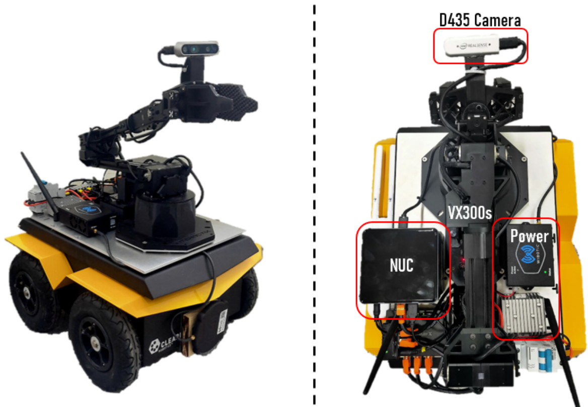
Figure 4.1: Medicine Delivery Robot. Perception, movement, grasping, and calculation functions were integrated on the Jackal, and it can shuttle between the ward and the pharmacy to complete handover and medicine delivery tasks.
