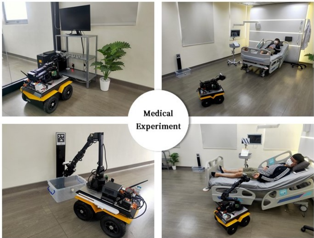
Figure 4.7: Upper left picture displays the Grasp action; the robot is grasping a small medicine cup. The upper right picture displays the Movement action, in which the robot delivers medicine cups. The lower right picture presents the Handover action, which is key focus of this thesis. The lower left picture presents the Placement of the medicine cup to recycle the medicine cup and complete the series of tasks.
