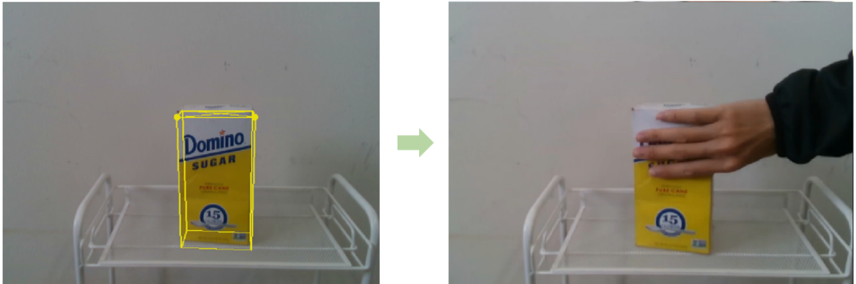
Figure 1.4: Handover occlusion will affect predict results. (The occlusion threshold is 44.5%)
