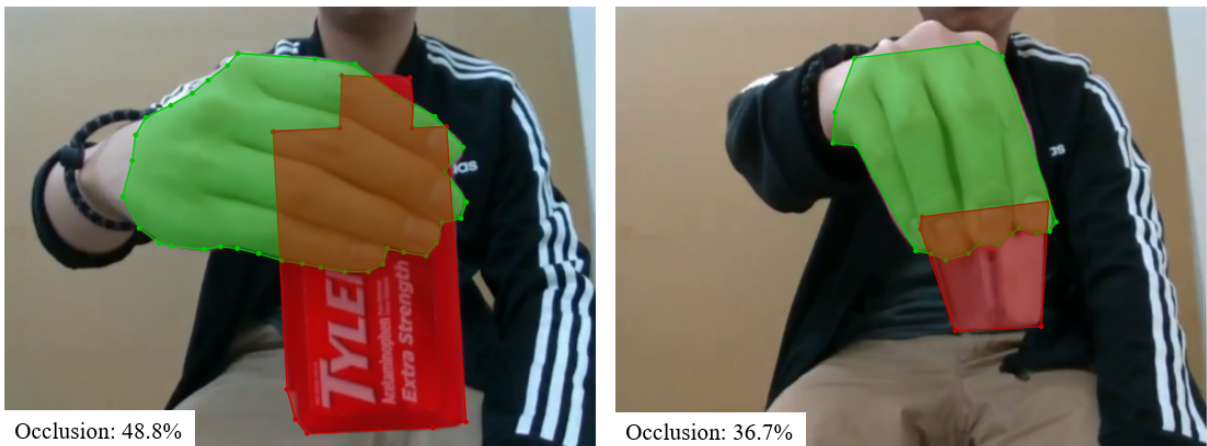
Figure 4.6: Example capture of the current frame of the grasp execution for labelling hand/object segmentation and estimating the occlusion ratio.
